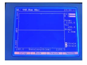
The spectrum measurement mode enables measurement parameters to be changed and post measurement tools to be accessed. The four options at the bottom of the screen allow the user to edit the scan settings, select the measurement mode, perform a post measurement search of the spectrum or apply a smoothing algorithm to the displayed scan. These options are selected with the corresponding function buttons.
