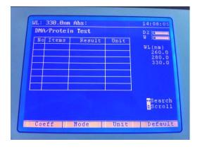
The DNA/Protein measurement mode enables measurement parameters to be changed. The four options at the bottom of the screen allow the user to edit the concentration calculation factors, select the measurement mode, select the units the of measurement and reset the modes settings to their default values. These options are selected with the corresponding function buttons.
