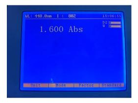
Insert the cuvette containing the blank solution into the reference position in the sample chamber and insert the cuvette containing the sample solution into the sample position. Close the instrument lid and the photometric result will be shown on the screen.
