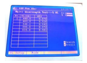
Insert a cuvette containing the sample to be analysed into the sample chamber and press the key below the sample measurement icon. The instrument will take a reading at each of the specified wavelengths the operating menu screen will then display the result of the selected measurement calculation and the photometric readings for each of the measured wavelengths.
