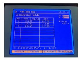
Once all standard solutions have been measured the new standard curve and curve equation will be shown.
