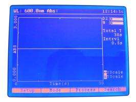
The kinetics enables measurement mode measurement parameters to be changed and post measurement tools to be accessed. The four options at the bottom of the screen allow the user to edit the kinetics run settings, select the measurement mode, perform a linear regression analysis on the data and perform a post measurement search of the scan's data These options are selected corresponding function buttons.
