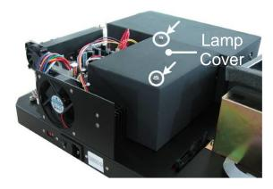
2. Unscrew the 2 screws on the top of the lamp chamber and remove the cover.
