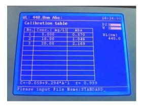
A standard curve can be saved to the instrument's internal memory to allow it to be recalled for future use.
