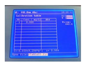
A standard curve can be opened from the instrument's internal memory to allow it to be re-used for sample quantification.
