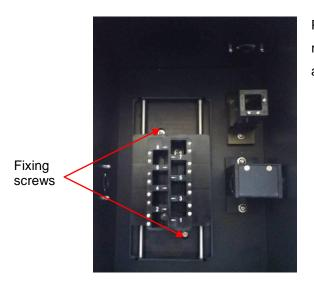
Place the accessory in the correct orientation and re-tighten the two fixing screws to fix the 8 cell accessory in place.
