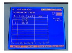
Insert the cuvette containing the blank solution into the reference position in the sample chamber and insert the cuvette containing the first standard solution into the sample position. Close the instrument lid and press the start/stop button. Once the measurement is complete the instrument will ask for the second standard solution to be inserted. Repeat the measurement procedure for each standard solution.
