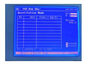
The quantitation measurement mode enables measurement parameters to be changed. The two options at the bottom of the screen allow the user to select the unit of measurement and edit the calibration standard settings. These options are selected with the corresponding function buttons.
