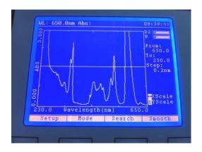
Insert a cuvette containing the blank solution into the reference position in the sample chamber and insert the cuvette containing the sample solution into the sample position. Close the instrument lid and press the Start/Stop key on the keypad. Once the measurement is complete the measured spectrum scan will be displayed on the screen.
