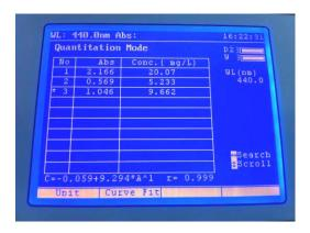
Ensure that a cuvette containing the blank solution is in the reference position in the sample chamber and insert the cuvette containing the sample solution into the sample position. Close the instrument lid and pres the Start/Stop key on the keypad. Once the measurement is complete the determined result will be displayed in the quantitation mode screen. Further samples can be measured in a similar manner.
