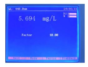
Remove the cuvette containing the blank solution and place a cuvette containing the sample to be measured in the sample chamber. Close the instrument lid and the concentration value will be shown on the screen.
