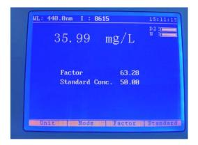
Remove the cuvette containing the standard sample and place a cuvette containing the sample to be measured in the sample chamber. Close the instrument lid and the calculated concentration value will be shown on the screen.
