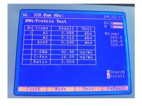
Ensure that a cuvette containing the blank solution is in the reference position in the sample chamber and insert the cuvette containing the sample solution into the sample position. Close the instrument lid and pres the Start/Stop key on the keypad. Once the measurement is complete the determined results will be displayed in the DNA/Protein mode screen. Further samples can be measured in a similar manner.
