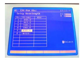
The measurement wavelengths of the selected measurement mode can be adjusted by pressing the function key below the WL Setup option or the GOTOλ key on the instrument keypad. The required wavelengths can be entered using the numerical keypad, pressing the Enter key to confirm each value. Further values can be added by moving to a new line with the down arrow key. Once all the required wavelengths have been entered press the ESC key to exit the wavelength selection screen.
