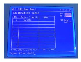
The user can manually enter the calibration curve constants by pressing the function key below the Params option. The user will be prompted to enter the constants that are required for the selected curve fit algorithm.
