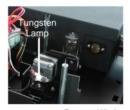
Whilst wearing cotton gloves remove the defective tungsten lamp and replace with a new one.
