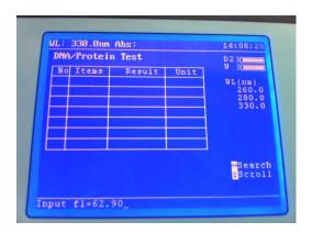
The measurement mode option can be selected by pressing the function key below the Coeff option.
