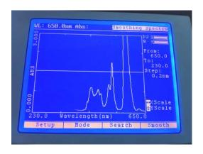
The measured spectrum scan can be smoothed by pressing the function key below the Smooth option.
