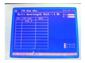
The multi-wavelength measurement mode enables measurement parameters to be changed. The two options at the bottom of the screen allow the user to edit the measurement wavelengths and change the measurement mode. These options are selected with the corresponding function buttons.
