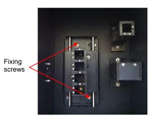
Unscrew the two fixing screws to undo the passive accessory. Lift out the passive accessory.
