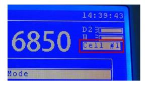
To activate the accessory press the Cell key on the instrument keypad. The indicated cell position will be highlighted on screen.
