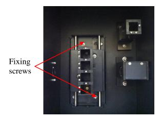
Unscrew the two fixing screws to undo the passive accessory. Lift out the passive accessory. To fit a different passive accessory place the accessory in the correct orientation and re-tighten the two fixing screws to fix in place.
