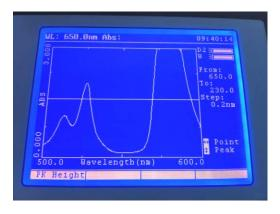
The photometric values of the measured spectrum can be viewed by pressing the function key below the Search option. The user can press the up and down arrow keys to move between the peaks in the scan that are above the threshold peak height. The user can alternatively press the left or right arrow keys to review each point in the scan in turn.
