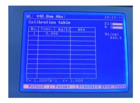
The quantitation table settings are accessed by pressing the function key below the Curve Fit option in the quantitation mode screen. Four new options are available in the quantitation table screen:
