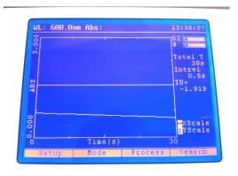
Insert a cuvette containing the blank solution into the reference position in the sample chamber and insert the cuvette containing the sample solution into the sample position. Close the instrument lid and press the Start/Stop key on the keypad. Once the measurement is complete the measured kinetics scan will be displayed on the screen.
