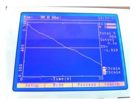
The instrument software allows the user to calculate the concentration of a substance from the difference between the photometric values at two time points in the displayed kinetics scan.
