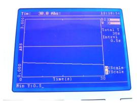
The instrument will display the full range scan after a measurement is complete. To change the displayed time range, press the left or right arrow keys. The start and end times can be entered using the numeric keypad. Press the Enter key to confirm. To change the displayed photometric range, press the up or down arrow keys. The minimum and maximum values can be entered using the numeric keypad. Press the Enter key to confirm.
