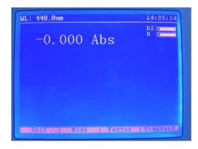
A zero calibration can be performed at the same wavelength at which the sample will be measured. With both the reference a sample positions empty and the sample chamber lid closed, press the 100%T/0Abs button to zero the instrument's photometric reading.
