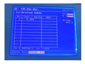
The curve fit algorithm can be selected by pressing the function key below the Method option. Four curve fit options are available:
