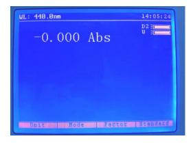
The photometrics measurement mode screen enables measurement parameters to be changed. The four options at the bottom of the screen allow the user to select the unit of measurement, the measurement mode, the concentration factor and the calibration standard's concentration. These options are selected with the corresponding function buttons.
