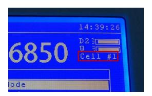
When the automatic 8 cell turret is installed the current cell position is indicated below the lamp status icons in the top right hand corner of the screen.
