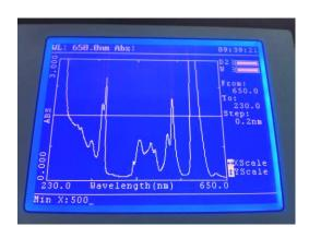
The instrument will display the full range scan after a measurement is complete. To change the displayed wavelength range, press the left or right arrow keys. The minimum and maximum display wavelengths can be entered using the numeric keypad. Press the Enter key to confirm. To change the displayed photometric range, press the up or down arrow keys. The minimum and maximum values can be entered using the numeric keypad. Press the Enter key to confirm.
