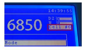
Each cell position is selected by pressing the corresponding digit on the numeric keypad. e.g. position 6 is selected by pressing the number 6 key on the instrument keypad. The instrument display will update to show the new automatic cell changer position.
