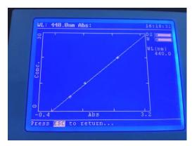
The standard curve can be viewed graphically by pressing the function key below the show curve option on the calibration table screen.
