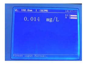
The concentration of a sample can be determined by using an appropriate multiplication factor with the measured photometric reading. A concentration factor can be entered by pressing the function button below the Factor option. The required factor can then be entered using the numerical keypad. Press the Enter key to confirm.
