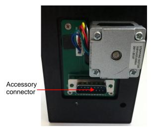
On the underside of the 8 cell accessory, locate the accessories power supply and communication connector.
