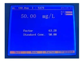
A calibration standard can be used to determine the concentration factor. Insert the cuvette containing the blank solution into the reference position in the sample chamber and insert the cuvette containing the standard solution into the sample position. Close the instrument lid. The concentration of the calibration standard is entered by pressing the function button below the Standard option. The concentration of the calibration standard can then be entered using the numerical
