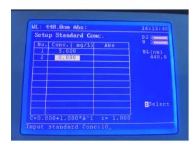
The user can edit the calibration curve data by pressing the function key below the Standard option. The user will be prompted to enter the concentration values for each standard. The values can be entered using the numerical keypad. Press the Enter key to confirm.
