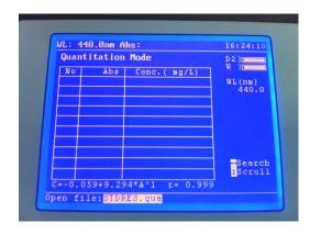
A result file can be opened from the instrument's internal memory.
