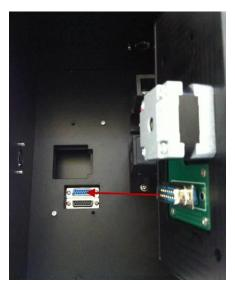
Take the 8 cell accessory and align the accessories connector with the instrument connection socket.
