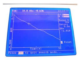
The photometric values of the measured kinetics scan can be viewed by pressing the function key below the Search option. The user can press the up and down arrow keys to review each point in the scan in turn.
